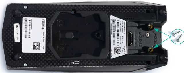
Location of the two M2.5x8 screws.
